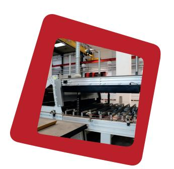
The machine is thought for the lamination of laminates up to a width of 2400mm.
